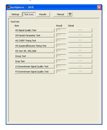
Click the [Droop Test] button in the dialog box. The Host Droop Test dialog box is displayed.
