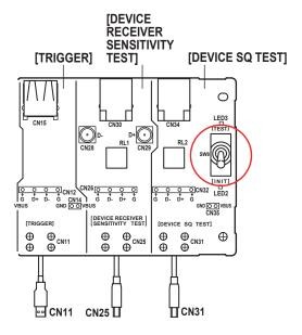
13. Click the [Next] button in the dialog box of the busXplorer-USB, click the [Enumerate Bus] button in the HS Electrical Test Tool .Then, select SUSPEND from the Port Control drop down menu and set the target port number in the HS Electrical Test Tool, then click [EXECUTE] button.
