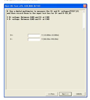
12. Click the [Next] button in the dialog box of the busXplorer-USB. Select TEST\_SE0\_NAK from Port Control drop down menu and set the target port number in the HS Electrical Test Tool, then click the [EXECUTE] button.
