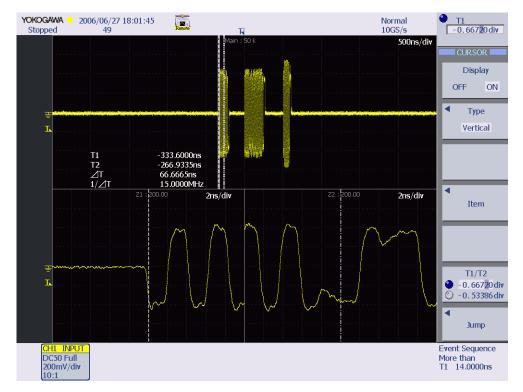
15. Confirm the Sync field of the 1st packet (EL\_21). Using the digital oscilloscope's zoom function, adjust the zoom position on the 1st packet. Then set the cursors of the digital oscilloscope on the start and the end points of the Sync field of the 1st packet. The Sync field must be 32 bits.
