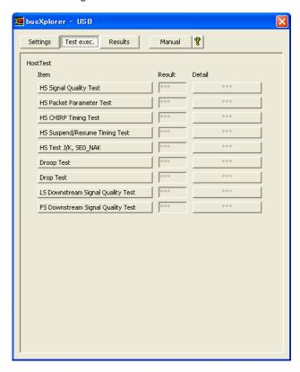
**2.** Click the **[FS Downstream Signal Quality Test]** button in the dialog box. The Host FS Downstream Signal Quality Test dialog box is displayed.
