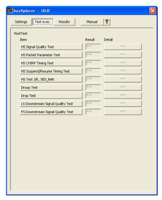
**2.** Click the **[LS Downstream Signal Quality Test]** button in the dialog box. The Host LS Downstream Signal Quality Test dialog box is displayed.
