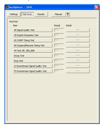
2. Click the [HS Signal Quality Test] button in the dialog box. The Host HS Signal Quality Test dialog box is displayed.
