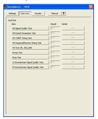
**2.** Click the **[HS Suspend/Resume Timing Test]** button in the dialog box. The Host HS Suspend/Resume Timing Test dialog box is displayed.
