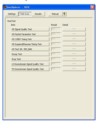
2. Click the [HS Packet Parameter Test] button in the dialog box. The Host HS Packet Parameter Test dialog box opens.
