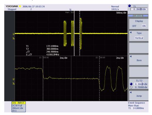
21. To measure the gap between packets (EL\_22), adjust zoom1 position to the end of the 2nd packet (from Device) and zoom2 position to the start of the 3rd packet (from Host). Then set the cursors on the end point of the 2nd packet in zoom1 and the start point of the 3rd packet in zoom2. The gap must be between 8bits and 192 bits.
