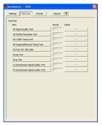
2. Click the [HS Test J/K, SE0\_NAK] button. The Host J/K, SE0\_NAK Test dialog box opens.
