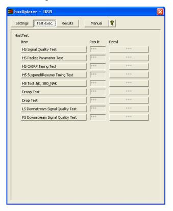
**2.** Click the **[Drop Test]** button in the dialog box. The Host Drop Test dialog box is displayed.
