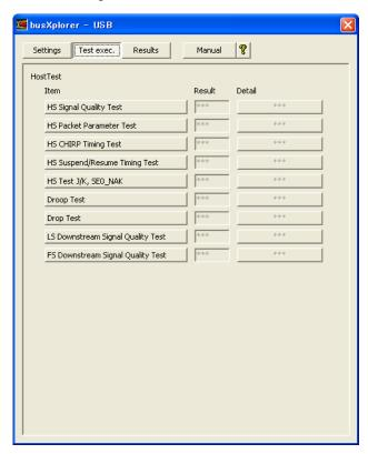
2. Click the [HS CHIRP Timing Test] button in the dialog box. The Host HS CHIRP Timing Test dialog box is displayed.
